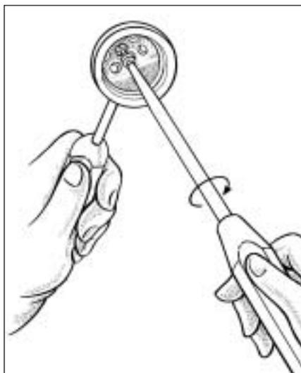
Fig. 16 Fixing the spikes.
